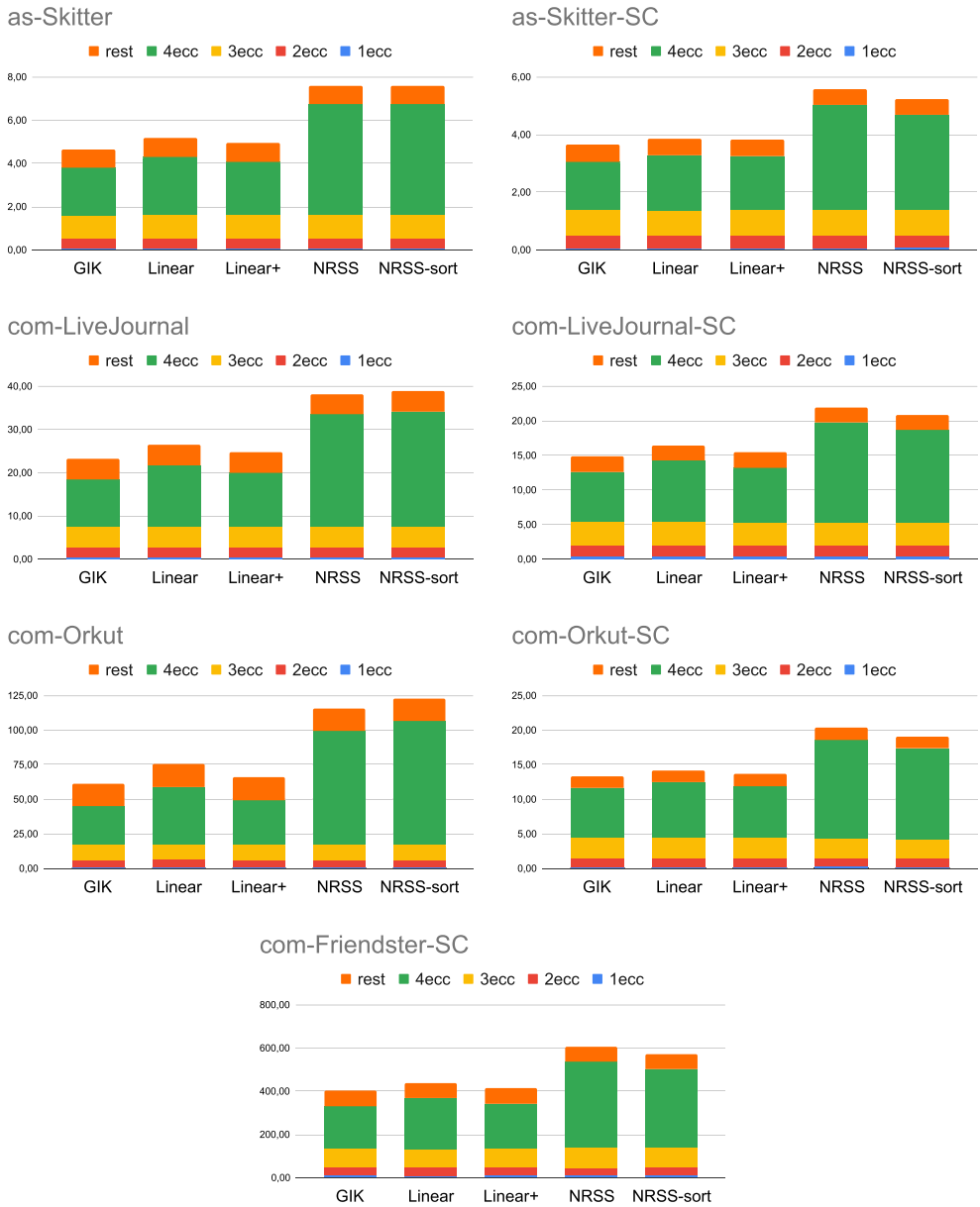
Fig. 7. Detailed running times for each part of the 4-edge-connected components algorithms on the last four real-world graphs of Table 1 and their sparse certificates. For each algorithm, we plot the running time for computing the (k - 1) -edge-cuts and the corresponding k -connected components for k \in \{1, 2, 3, 4\} .
