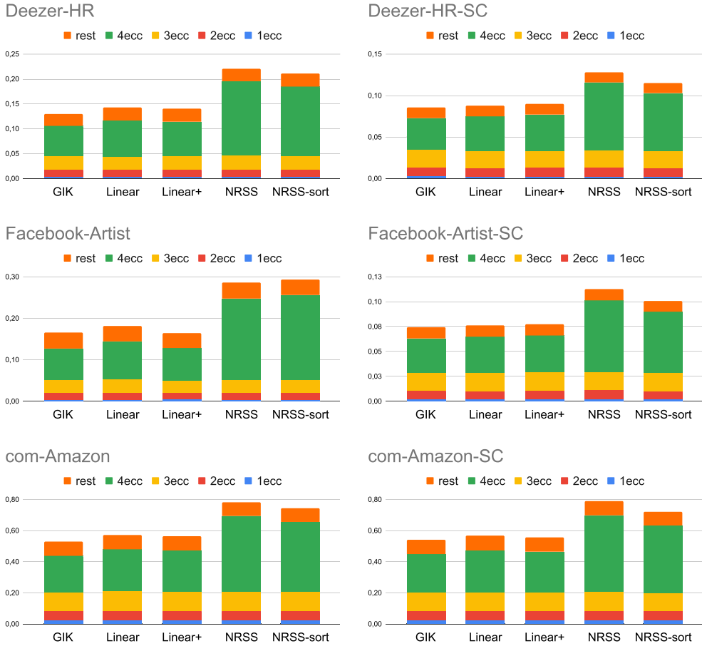
Fig. 5. Detailed running times for each part of the 4-edge-connected components algorithms on the first three real-world graphs of Table 1 and their sparse certificates. For each algorithm, we plot the running time for computing the (k - 1) -edge-cuts and the corresponding k -connected components for k \in \{1, 2, 3, 4\} .
